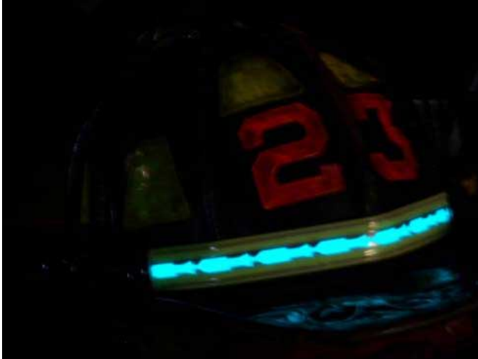
(3) The EL illuminated compared with the photoluminescence and other reflective materials on the helmet. Click to enlarge
